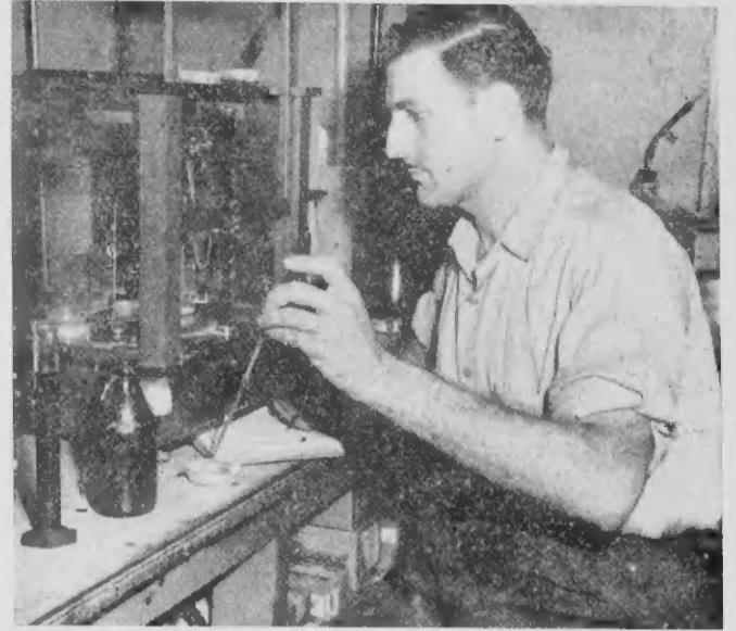
The aloe plant absorbs different quantities of water according to the rainfall. In the laboratory of the factory, a sample of the aloe juice is being tested for water content.
